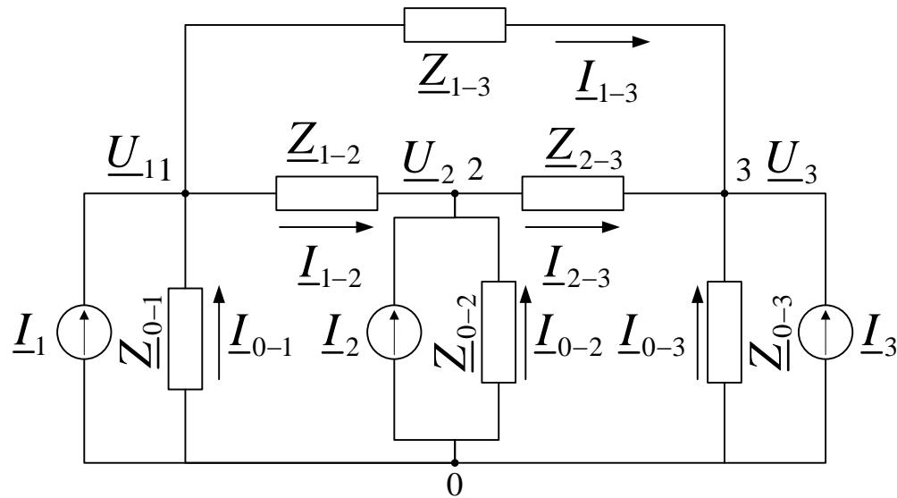
$$\underline{I}_1 = -\underline{I}_{0-1} + \underline{I}_{1-2} + \underline{I}_{1-3} = -\frac{\underline{U}_0 - \underline{U}_1}{\underline{Z}_{0-1}} + \frac{\underline{U}_1 - \underline{U}_2}{\underline{Z}_{1-2}} + \frac{\underline{U}_1 - \underline{U}_3}{\underline{Z}_{1-3}}$$
