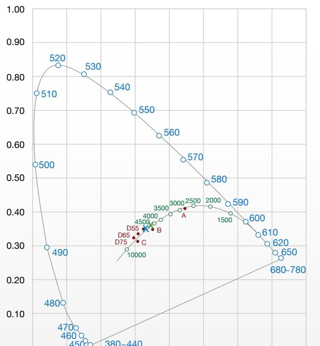
**Fig.18** xy chromaticity diagram comparing the colour temperature of an LED white and Natural White Fluorescent
