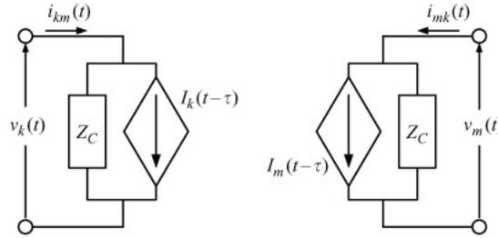
Figure 4.9: Equivalent two-port network for a lossless line
