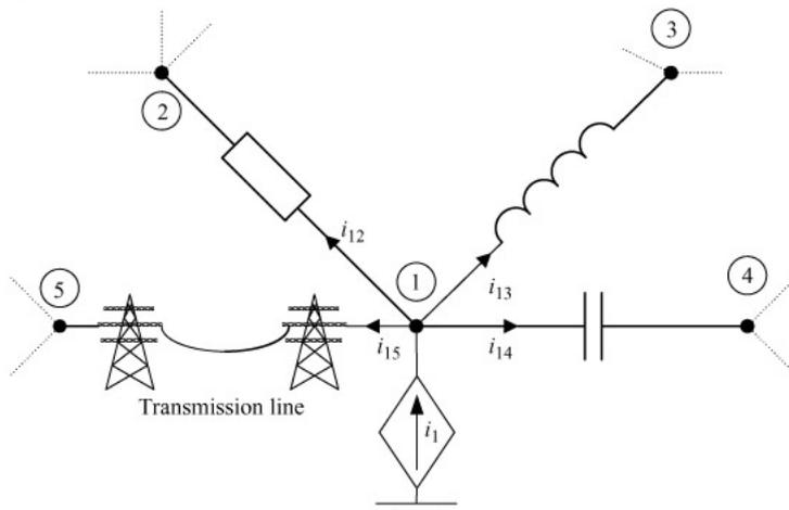
Figure 4.10: Node 1 of an interconnected circuit
